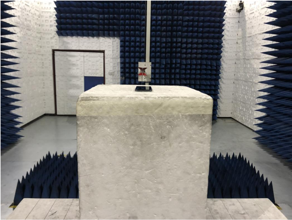
RADIATED EMISSION TEST SETUP ABOVE 1GHZ
