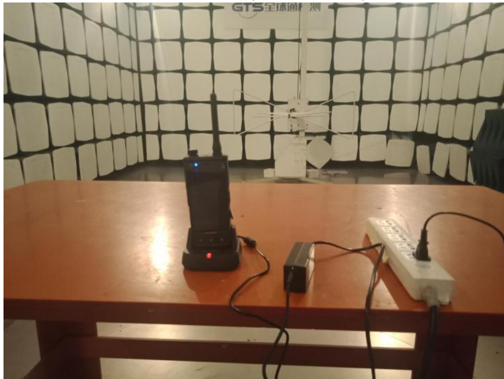
Radiated Emission(30MHz -1000MHz)
