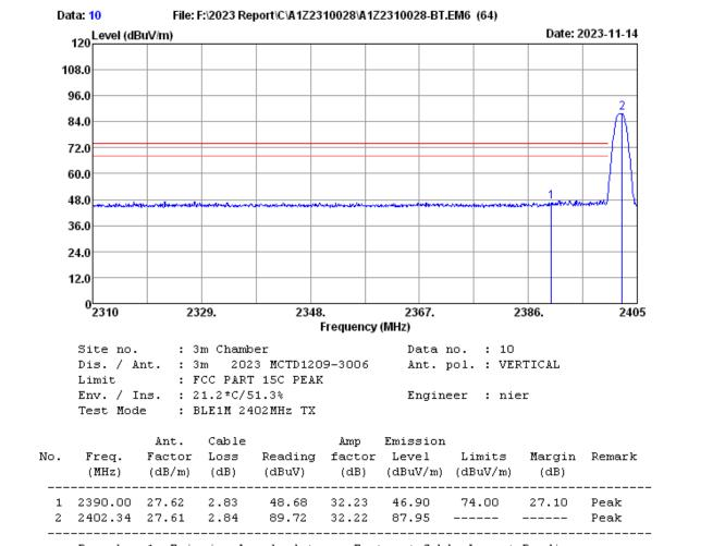
Remarks: 1. Emission Level= Antenna Factor + Cable Loss + Reading -Amp factor.
