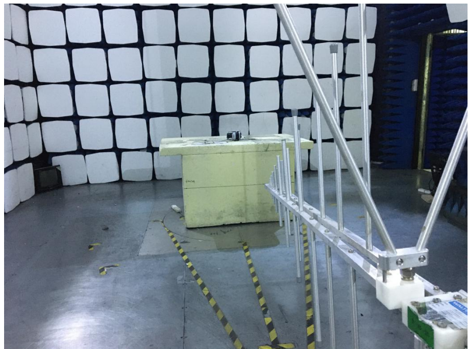
Radiation Emission Test Setup (30MHz to 1GHz)
