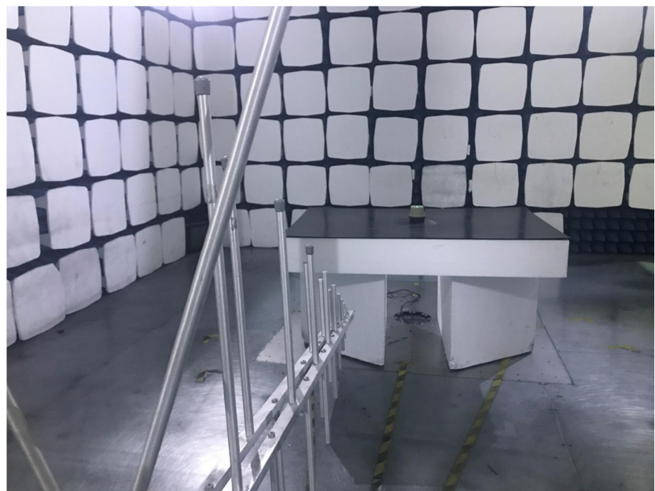
Radiation Emission Test Setup (30MHz to 1GHz)
