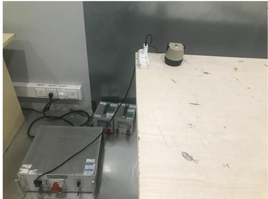
Conducted Emission Test Setup
