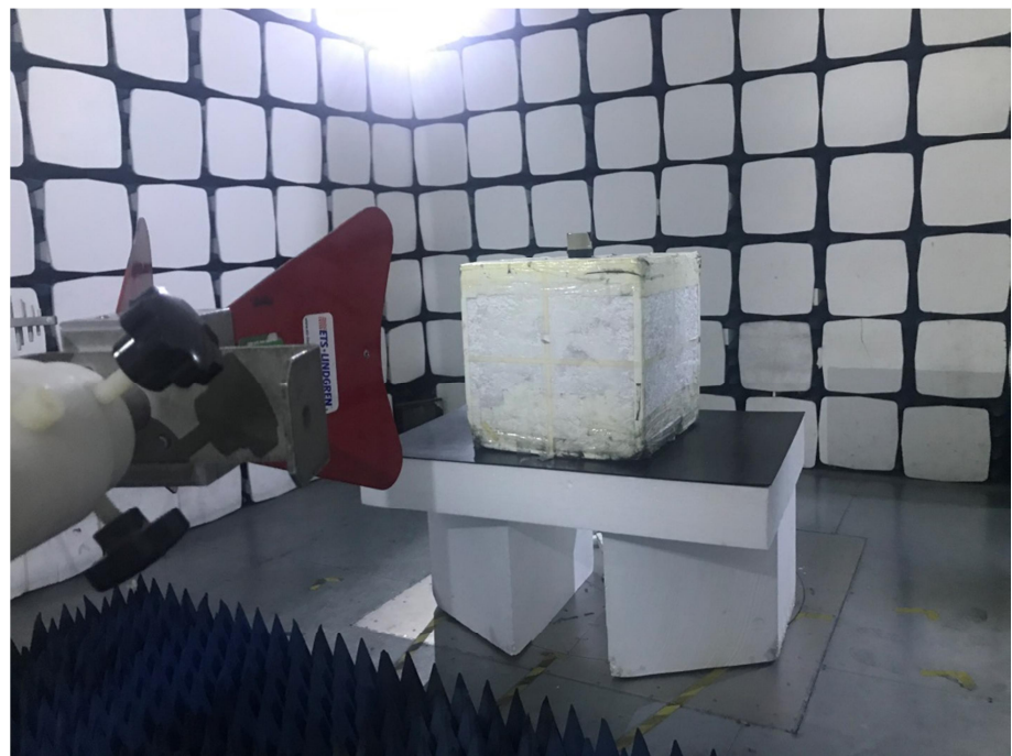
Radiation Emission Test Setup (1GHz to 18GHz)
