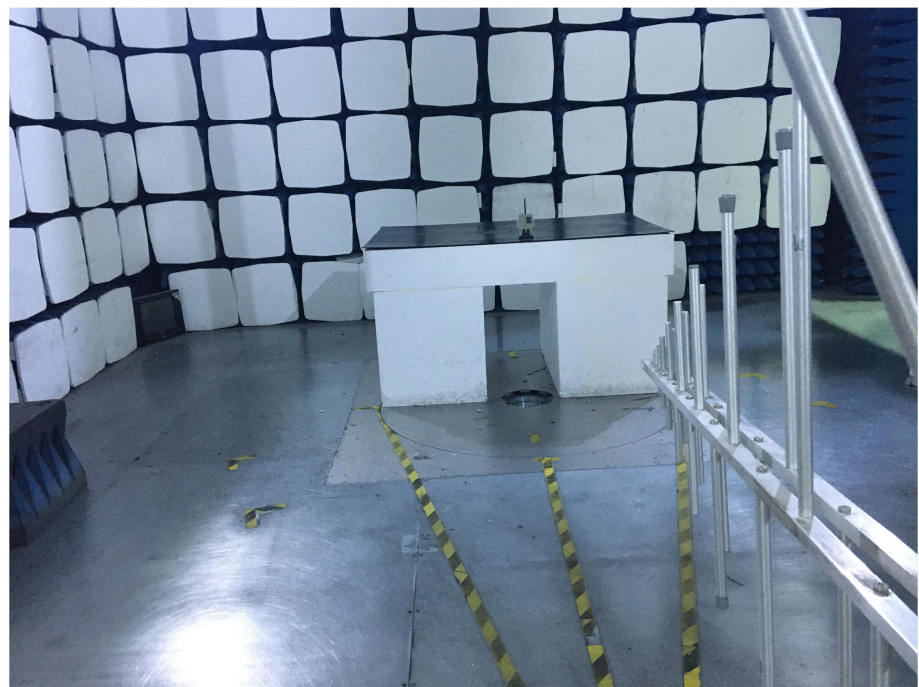
Radiation Emission Test Setup (30MHz to 1GHz)
