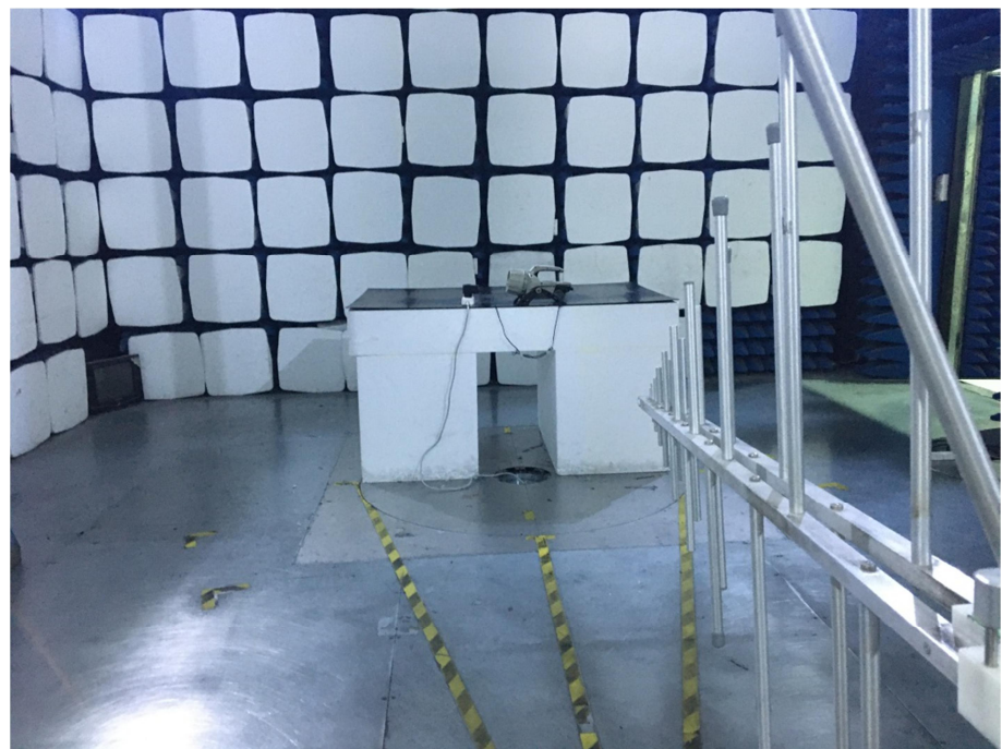
Radiation Emission Test View(30MHz to 1GHz)
