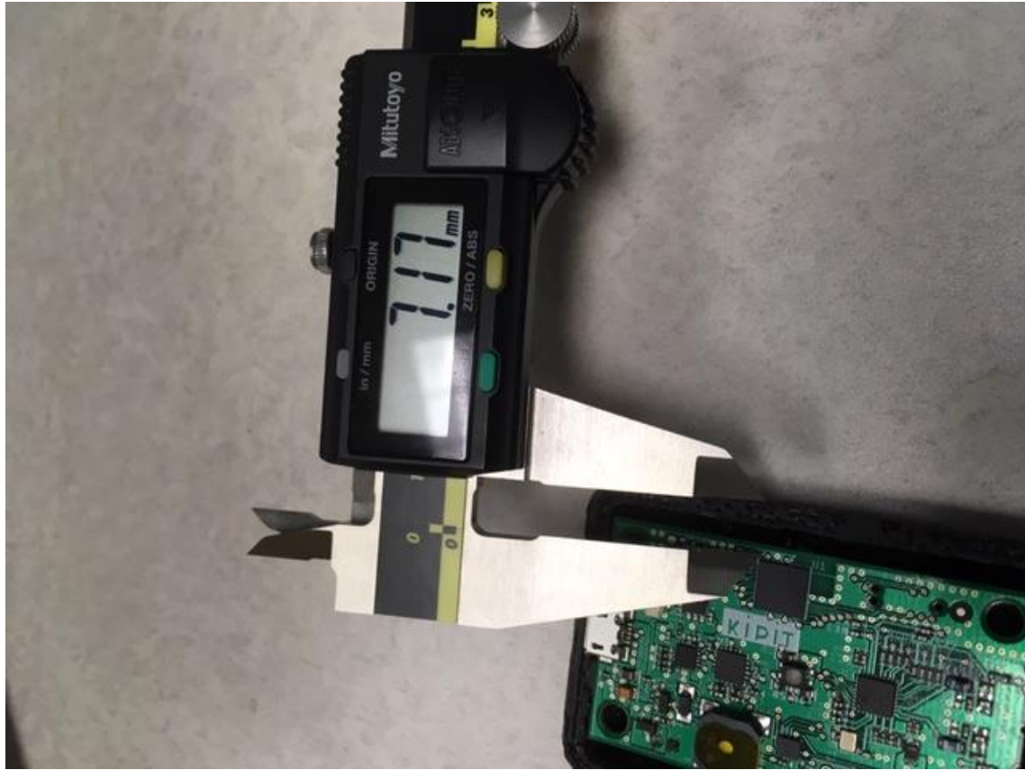
7.17 mm separation from module to side of case
