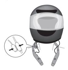
**Note:** The microphone connector has a special shape which allows the microphone to be connected in one way only.
