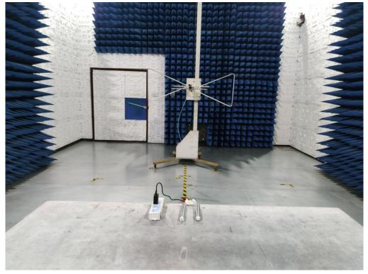
RADIATED EMISSION TEST SETUP ABOVE 1GHZ
