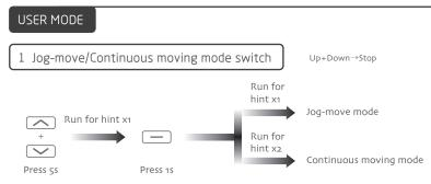
Note: In the jog-move mode, short press up/down button 2s to loosen, the motor is jog-move to run; If long press more than 2s, the motor run continuously, release the button, the motor stops running; In the continuous moving mode, long press up/down button, the motor runs continuously, release the button, the motor stops running.
