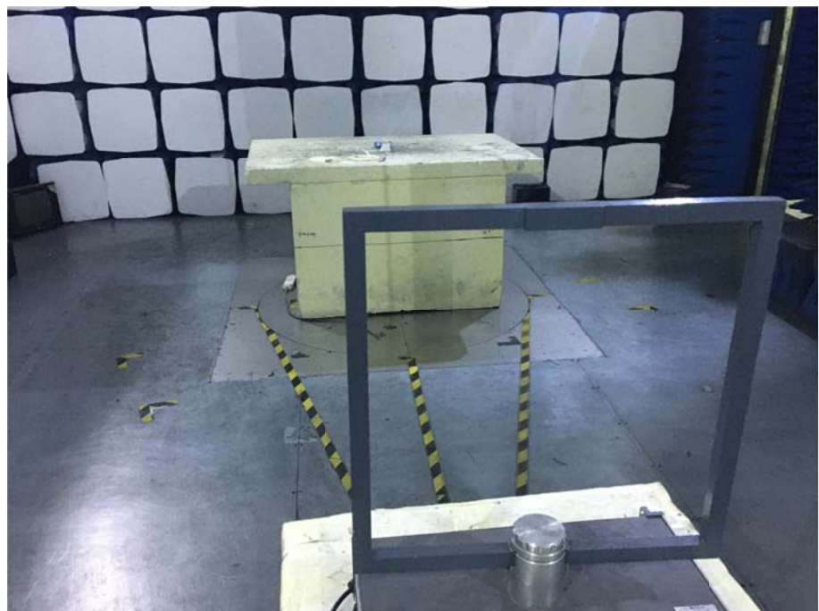
Radiation Emission Test Setup (Below 30MHz)
