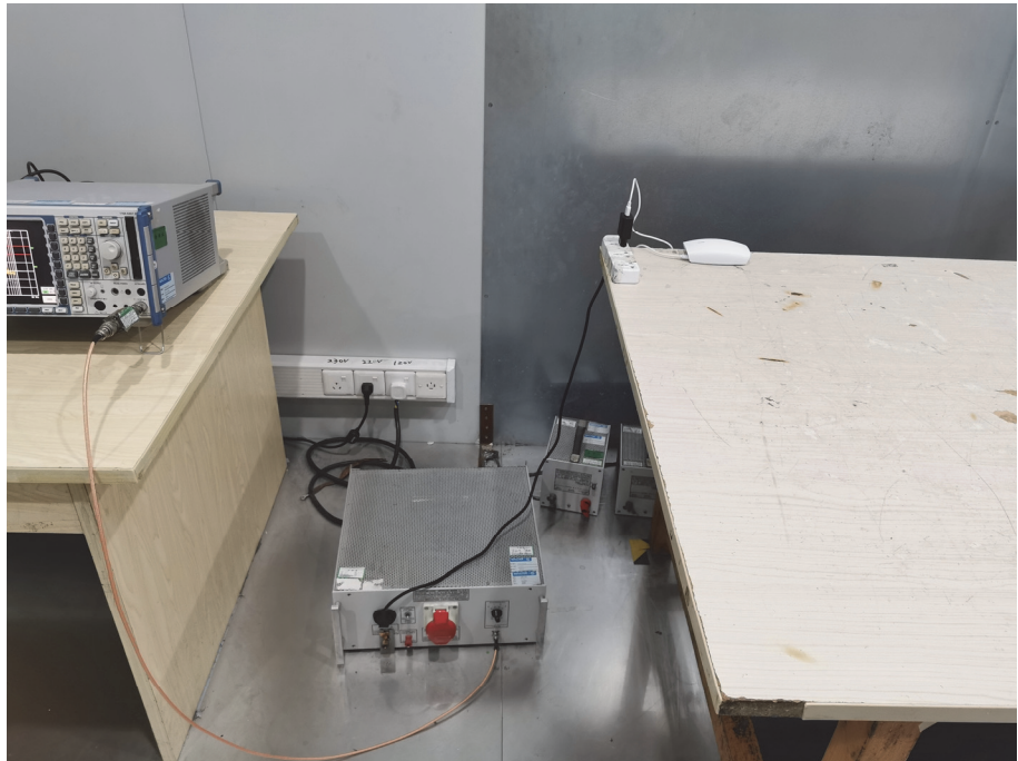
Conducted Emission Test Setup
