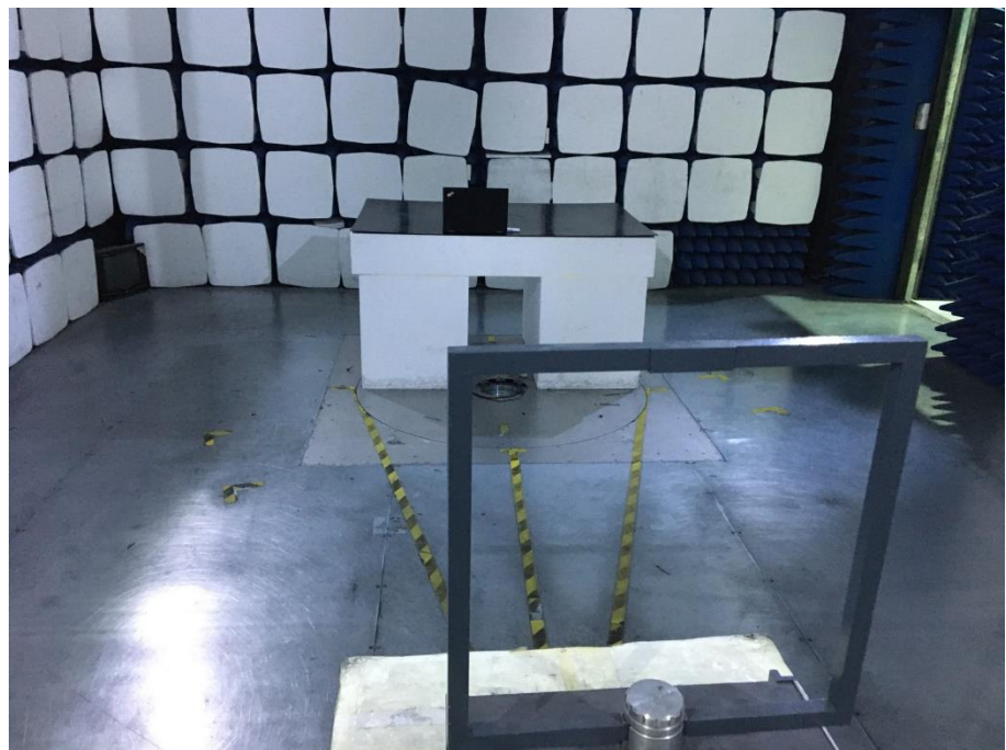
Radiation Emission Test Setup (Below 30MHz)
