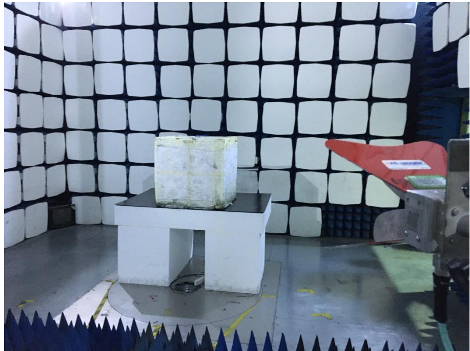
Radiation Emission Test Setup (1GHz to 18GHz)
