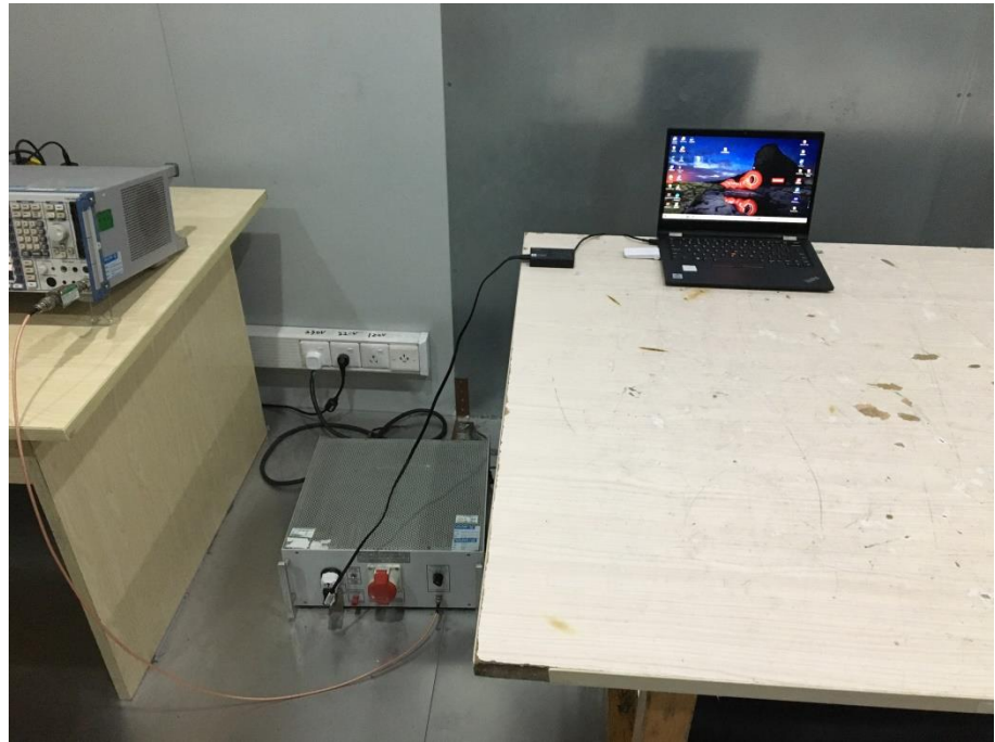
Conducted Emission Test Setup
