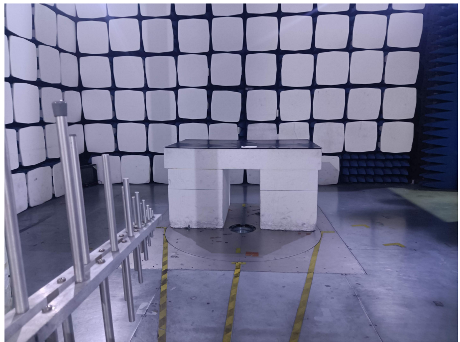
Radiation Emission Test Setup (30MHz to 1GHz)
