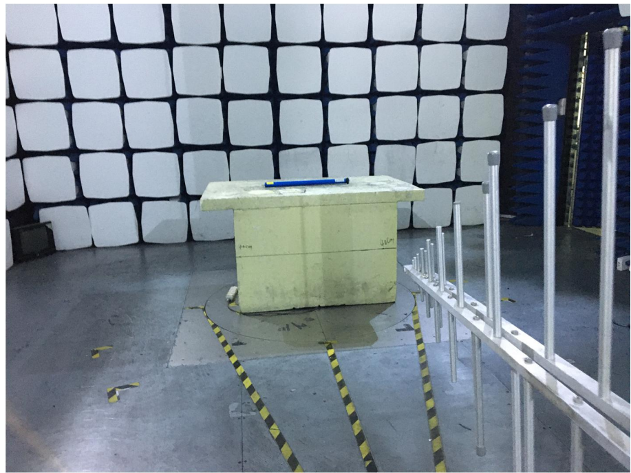
Radiation Emission Test Setup (30MHz to 1GHz)
