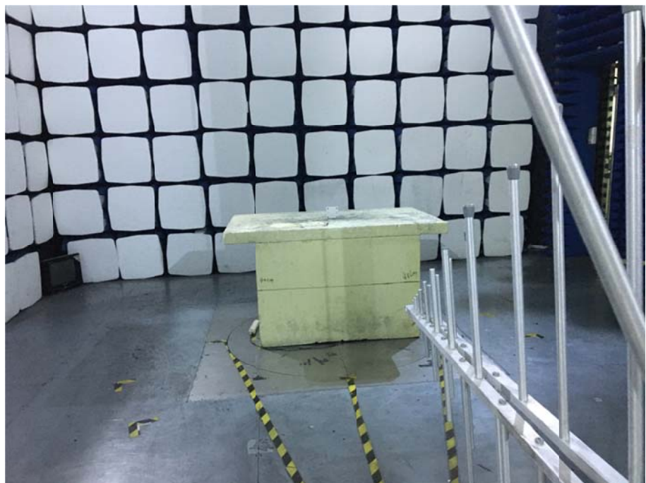
Radiation Emission Test Setup (30MHz to 1GHz)
