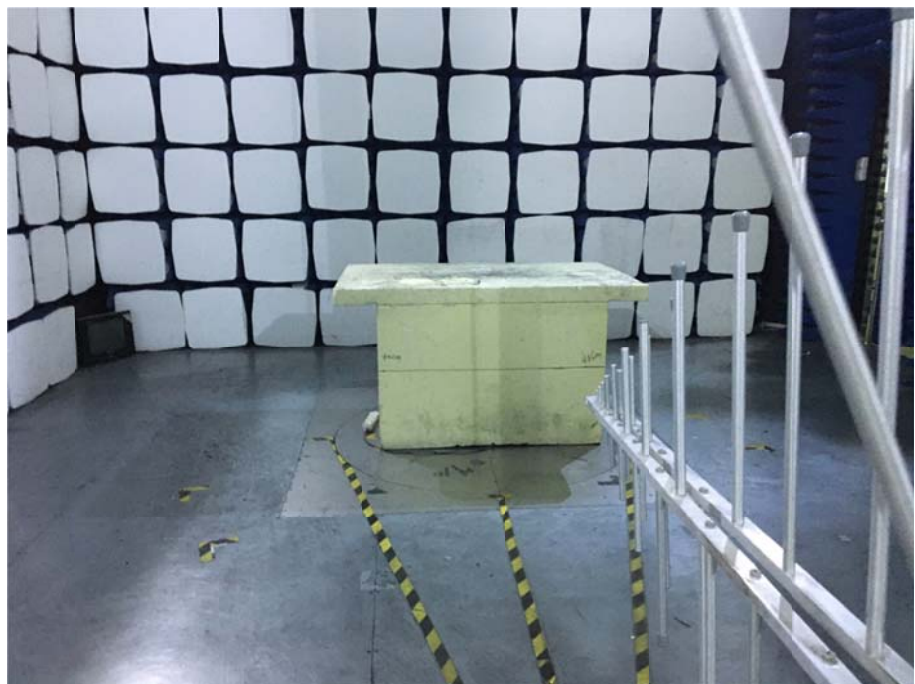
Radiation Emission Test Setup (30MHz to 1GHz)
