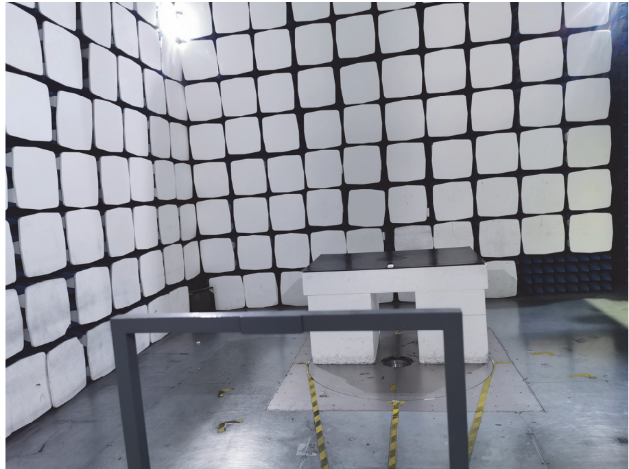
Radiation Emission Test Setup (Below 30MHz)
