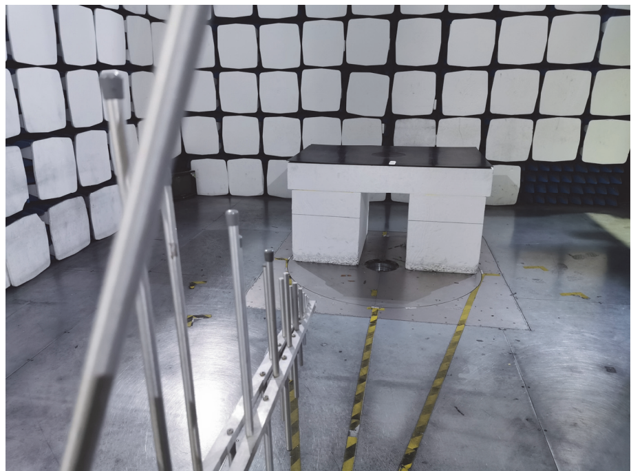
Radiation Emission Test Setup (30MHz to 1GHz)
