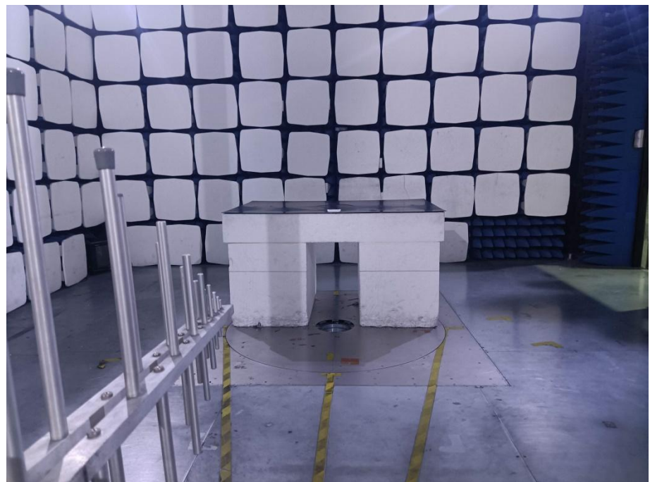
Radiation Emission Test Setup (30MHz to 1GHz)
