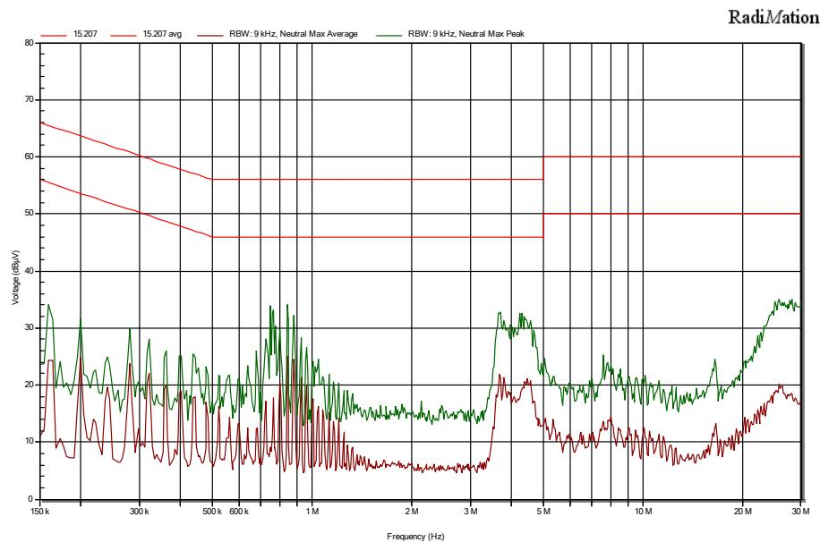
Note: the upper trace is to be compared with the upper limit line and the lower trace with the lower limit line.
