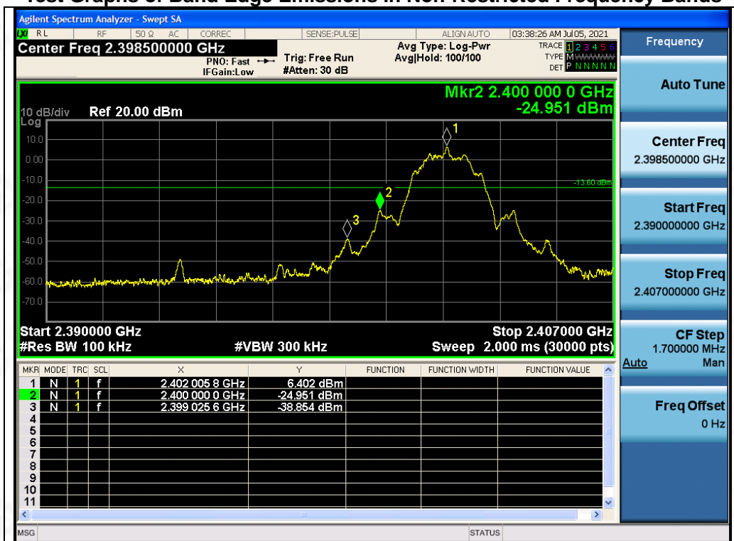
Test_Graph_LE2M_ANT1_2402_2Mbps_Lower Band Edge Emissions
