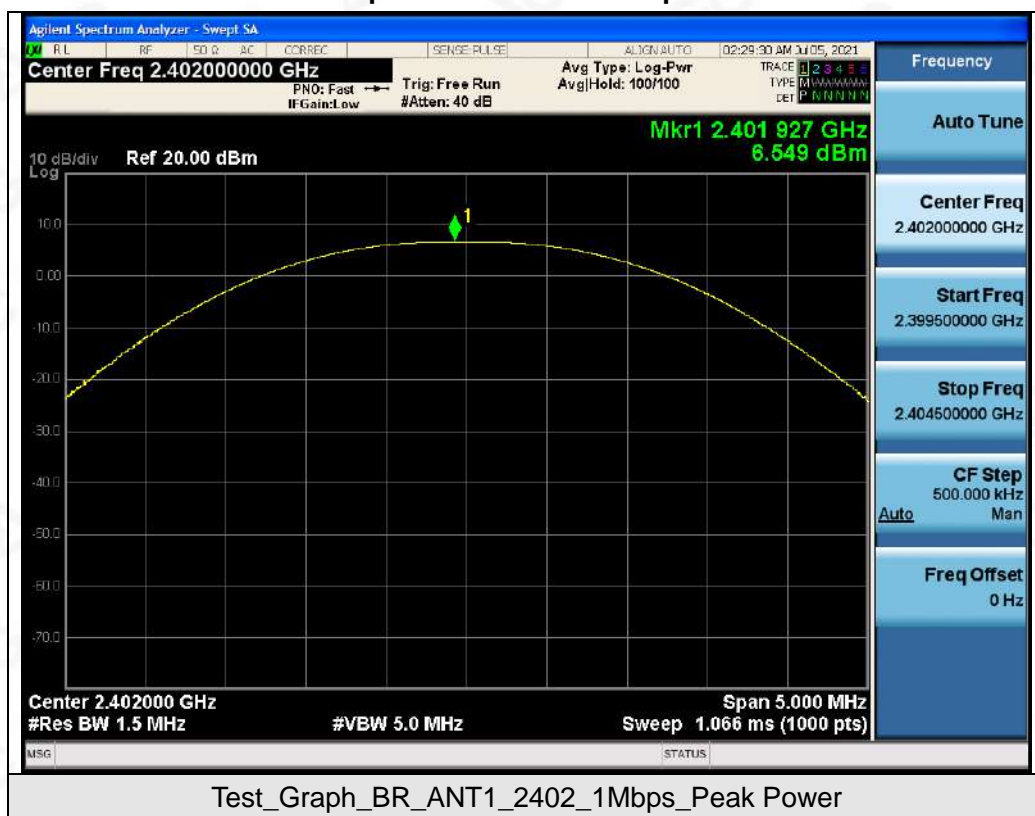
Test Graphs of Conducted Output Power
