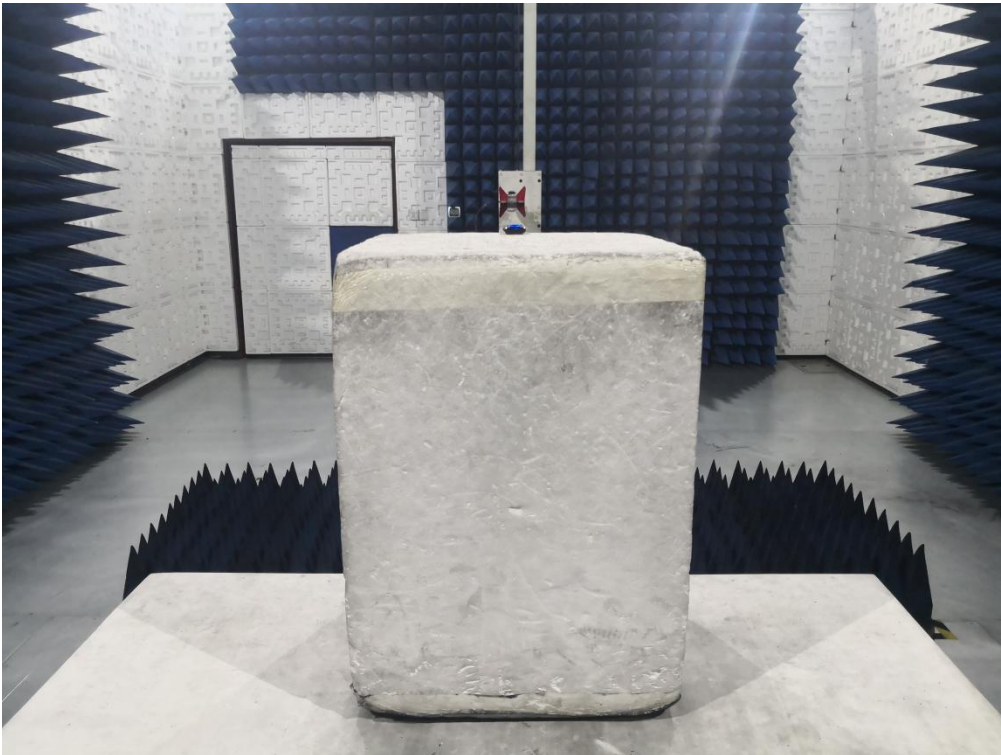
RADIATED EMISSION TEST SETUP ABOVE 1GHz
