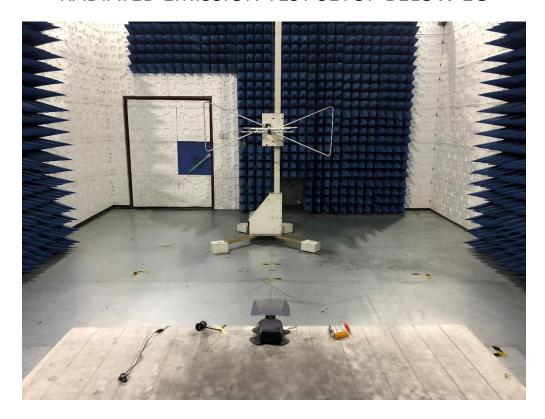
**RADIATED EMISSION TEST SETUP ABOVE 1G**
