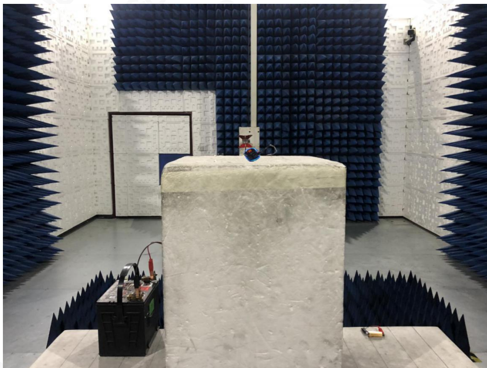
RADIATED EMISSION TEST SETUP ABOVE 1G
