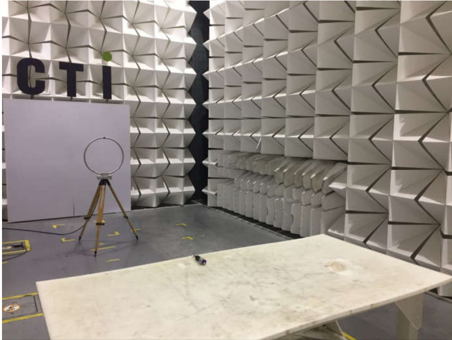
Radiated spurious emission Test Setup-1(Below 30MHz)
