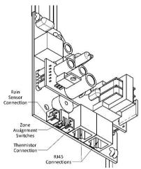
Each zone must be controlled by the MAXXFan PC Board. This board is located above the MAXXFan control plate. When installing the system, the MAXXFan PC Board must be set according to which zone the MAXXFan is to control.
