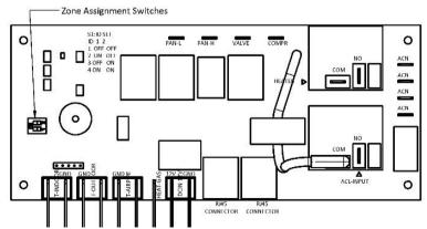
Each zone must be controlled by an upper unit control board. When installed, this board is located in the return air plenum of the rooftop unit. When installing the system, the upper unit control board must be set
