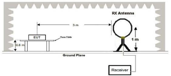
(2) Radiated Emission Test-Up Frequency 30MHz~1GHz
