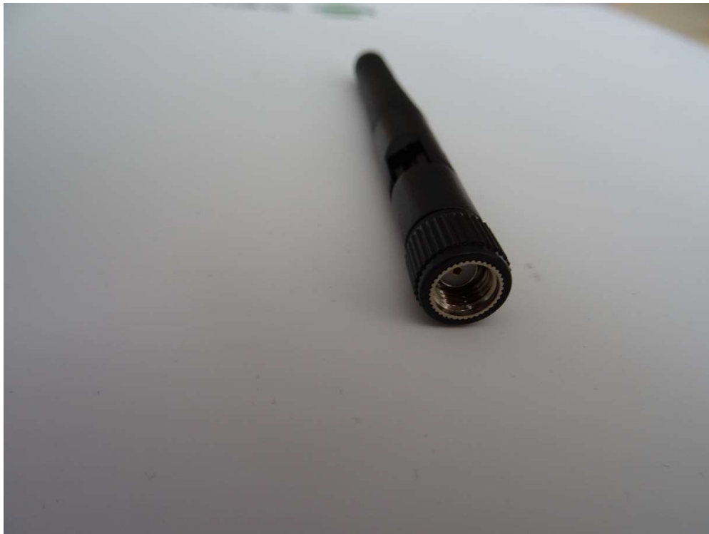
Photograph 5: antenna RP-SMA connector
