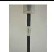
**Construction:** Symmetrical design with triangular core Built-in shielding against static charges
