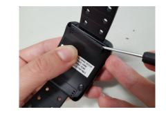
• Finally, remove the strap by placing the removal tool on the core of ActiveTrack, pressing firmly and then taking each strap end out of the core
