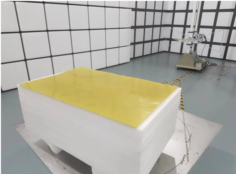
Photo of Radiated Emission Measurement (Above 1G)
