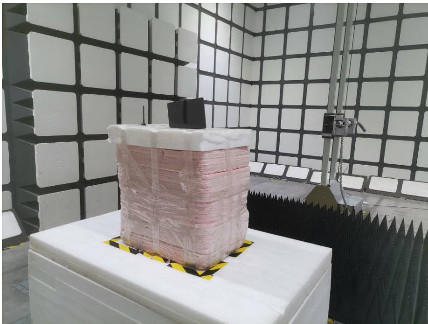
Radiated Emissions View (Above 1 GHz) – TX
