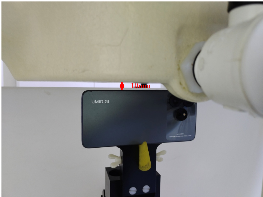
Body Right Setup Photo (10mm)
