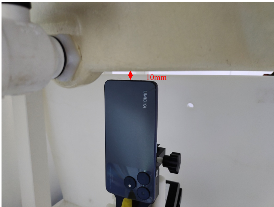
Body Bottom Setup Photo (10mm)
