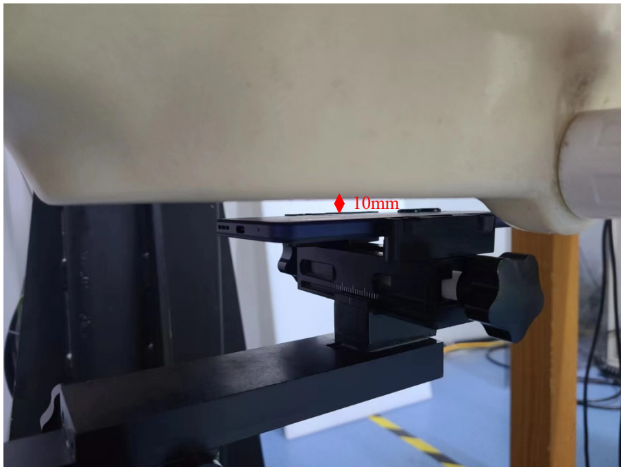
Body (Worn) Back Setup Photo (10mm)
