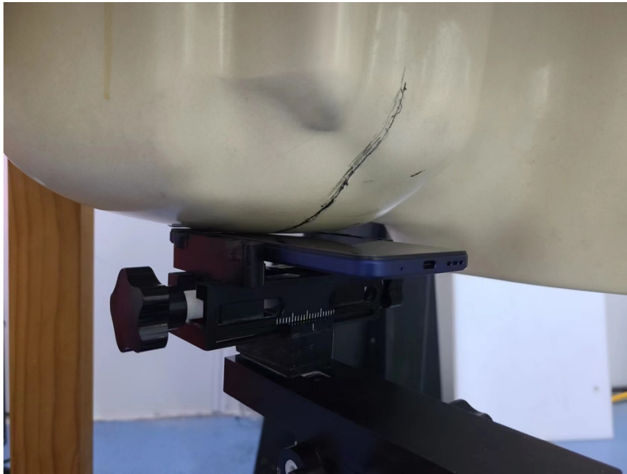
Head Right Tilt Setup Photo (0mm)
