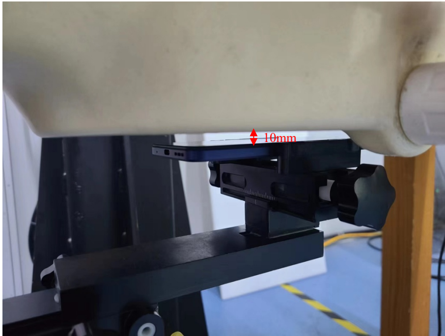
Body (Worn) Back Setup Photo (10mm)
