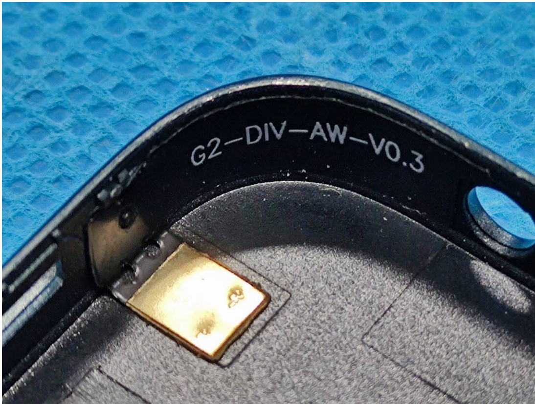
WWAN Main Antenna (TX Band: GSM 850, WCDMA B5, LTE B5/7/12/41)
