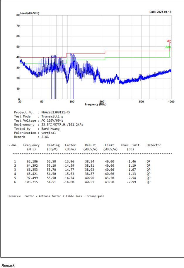
Level = Reading + Factor Factor = Antenna factor + Cable loss – Amplifier gain Over Limit = Level – Limit
