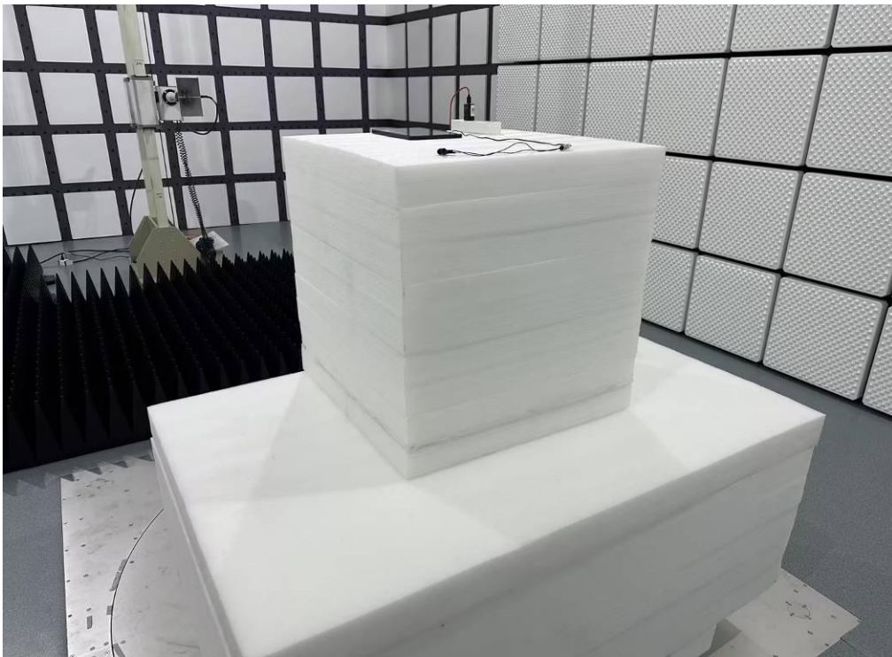
Photo of Radiated Emission Measurement (Above 1G)
