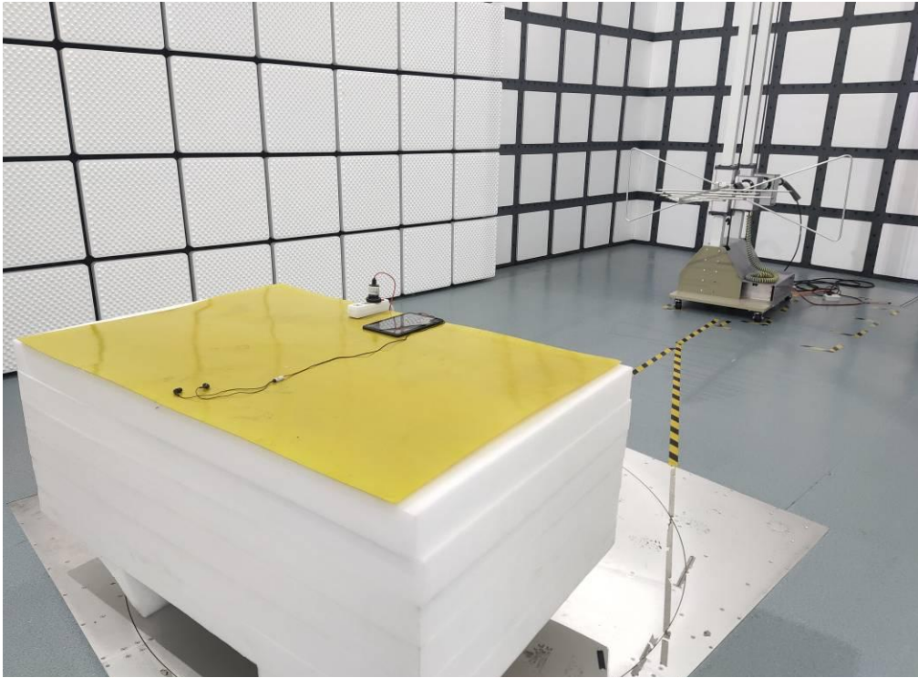
Photo of Radiated Emission Measurement (Above 1G)
