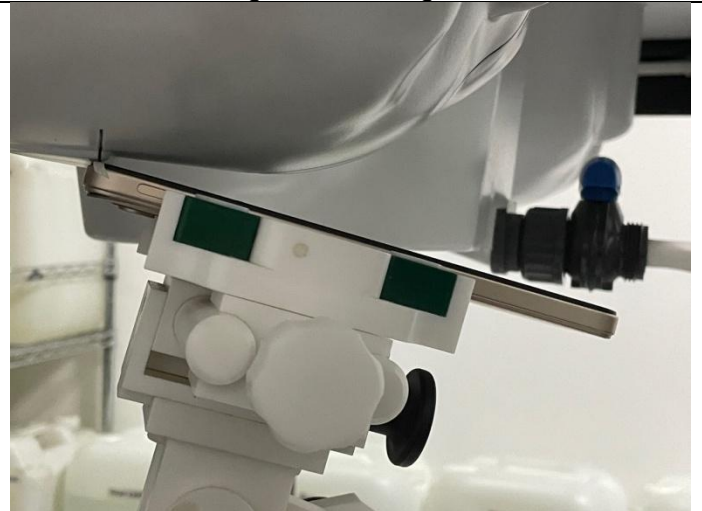
Back Side (Separation distance of 10mm)
