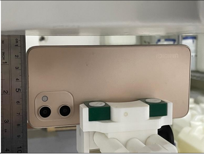
Top Side (Separation distance of 10mm)
