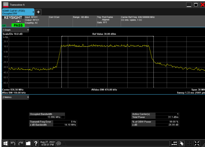
n5_15MHz_15kHz_836.5MHz_DFT-s-OFDM PI/2 BPSK_RB75@0
