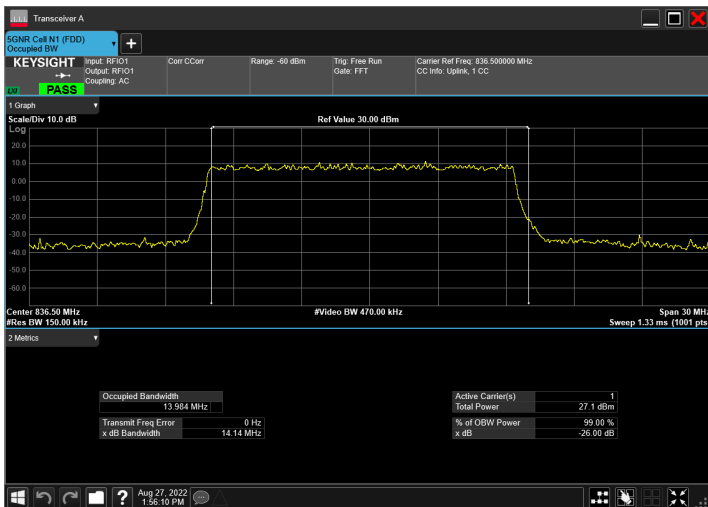
DC_2A_n5A_10MHz|15MHz_15kHz_1880MHz|836.5MHz_QP SK|DFT-s-OFDM 256 QAM_RB1@50|RB75@0
