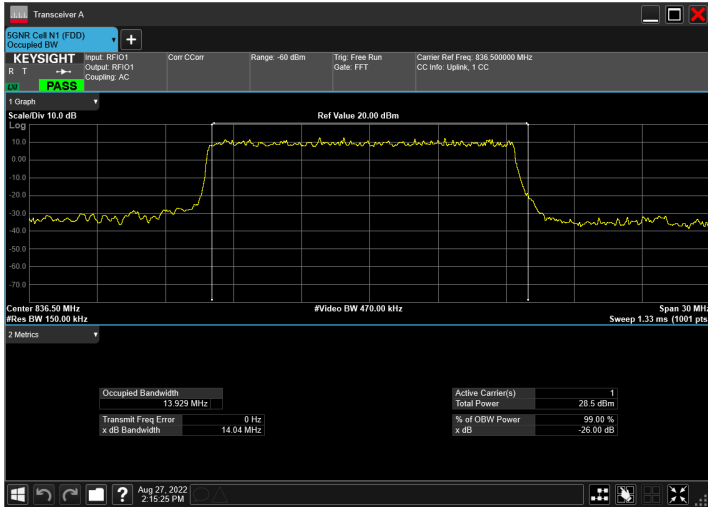
DC_2A_n5A_10MHz|15MHz_15kHz_1880MHz|836.5MHz_QP SK|DFT-s-OFDM PI/2 BPSK_RB1@50|RB75@0
