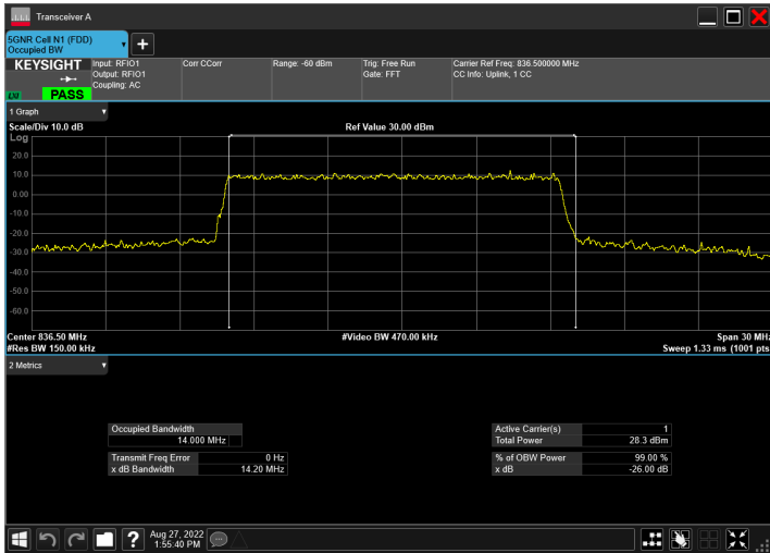
DC_2A_n5A_10MHz|15MHz_15kHz_1880MHz|836.5MHz_QP SK|DFT-s-OFDM 16 QAM_RB1@50|RB75@0
