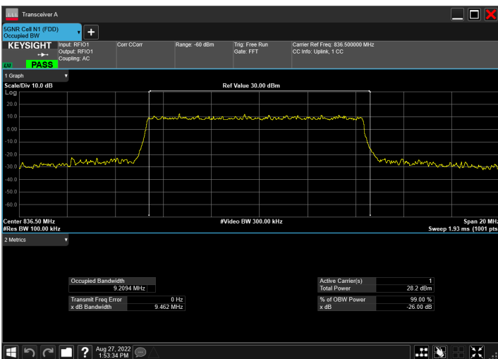
DC_2A_n5A_10MHz|10MHz_15kHz_1880MHz|836.5MHz_QP SK|CP-OFDM 64 QAM_RB1@50|RB52@0
