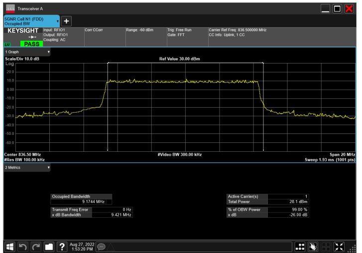
DC_2A_n5A_10MHz|10MHz_15kHz_1880MHz|836.5MHz_QP SK|CP-OFDM 16 QAM_RB1@50|RB52@0
