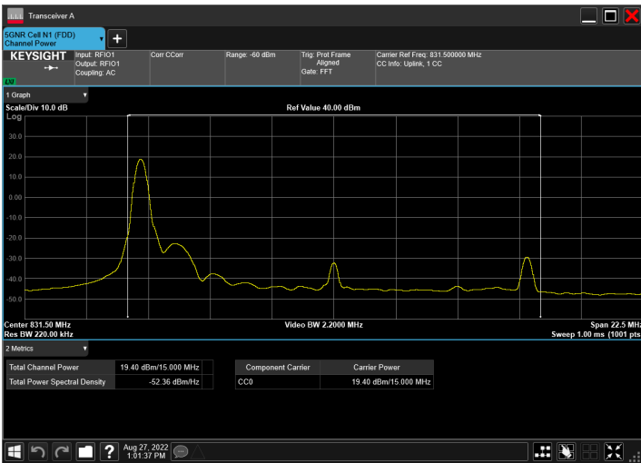
DC_2A_n5A_10MHz|15MHz_15kHz_1855MHz|831.5MHz_QP SK|DFT-s-OFDM QPSK_RB1@0|RB1@0
