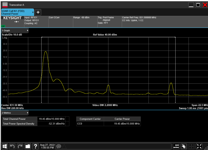
DC_2A_n5A_10MHz|15MHz_15kHz_1855MHz|831.5MHz_QP SK|DFT-s-OFDM PI/2 BPSK_RB1@0|RB1@0
