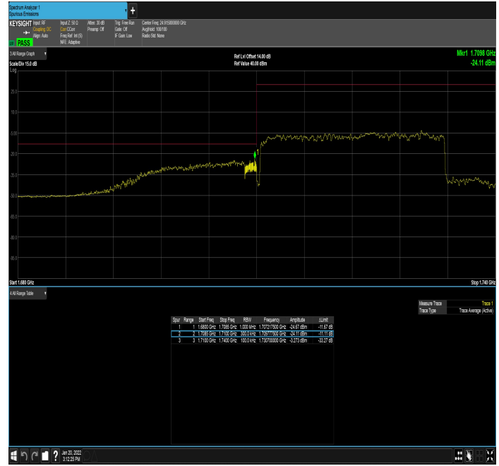
DC_12A_n66A_10MHz|25MHz_15kHz_704MHz|1722.5 MHz_DFT-s-OFDM QPSK_RB0|RB128@0
