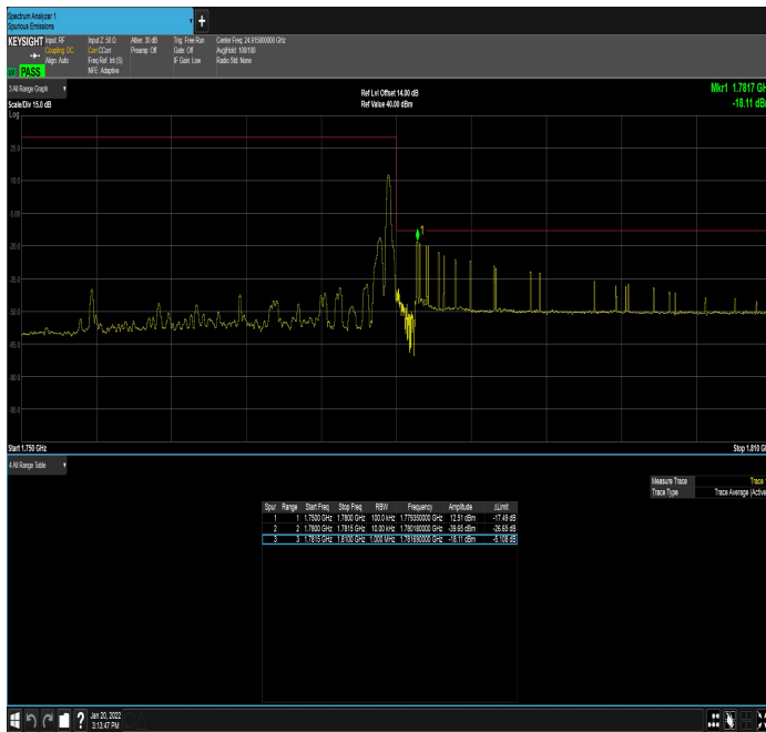
DC_12A_n66A_10MHz|25MHz_15kHz_711MHz|1767.5 MHz_DFT-s-OFDM QPSK_RB0|RB1@132
