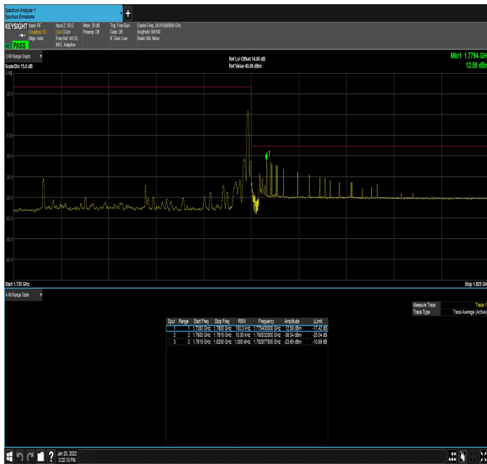
DC_12A_n66A_10MHz|40MHz_15kHz_711MHz|1760M Hz_DFT-s-OFDM QPSK_RB0|RB1@215
