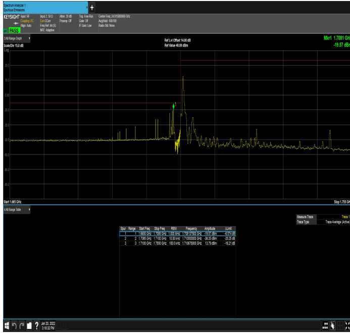
DC_12A_n66A_10MHz|40MHz_15kHz_704MHz|1730M Hz_DFT-s-OFDM QPSK_RB0|RB1@0
