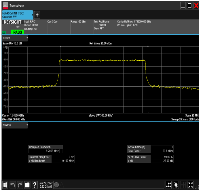
n66_10MHz_15kHz_1745MHz_CP-OFDM QPSK_RB52@0
