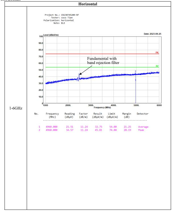
Listed with the worst harmonic margin test plot (BLE 1Mbps high channel) Horizontal:
