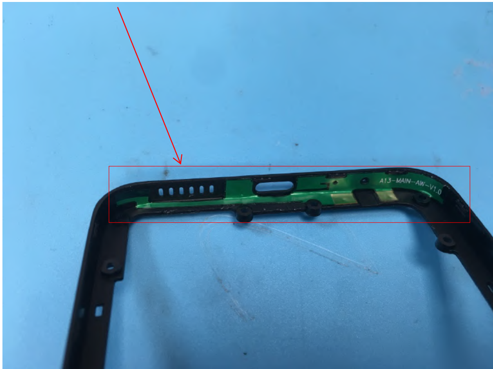
WWAN Aux Antenna (GSM1900, WCDMA B2, LTE B2/B41 TX)
