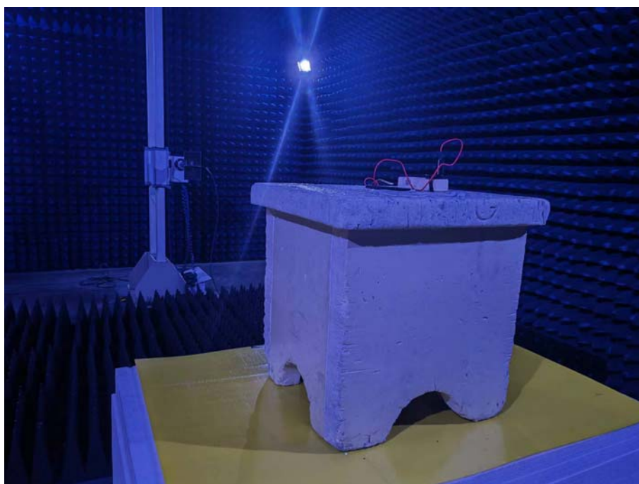
Photo of Radiated Emission Measurement (Above 1GHz)
