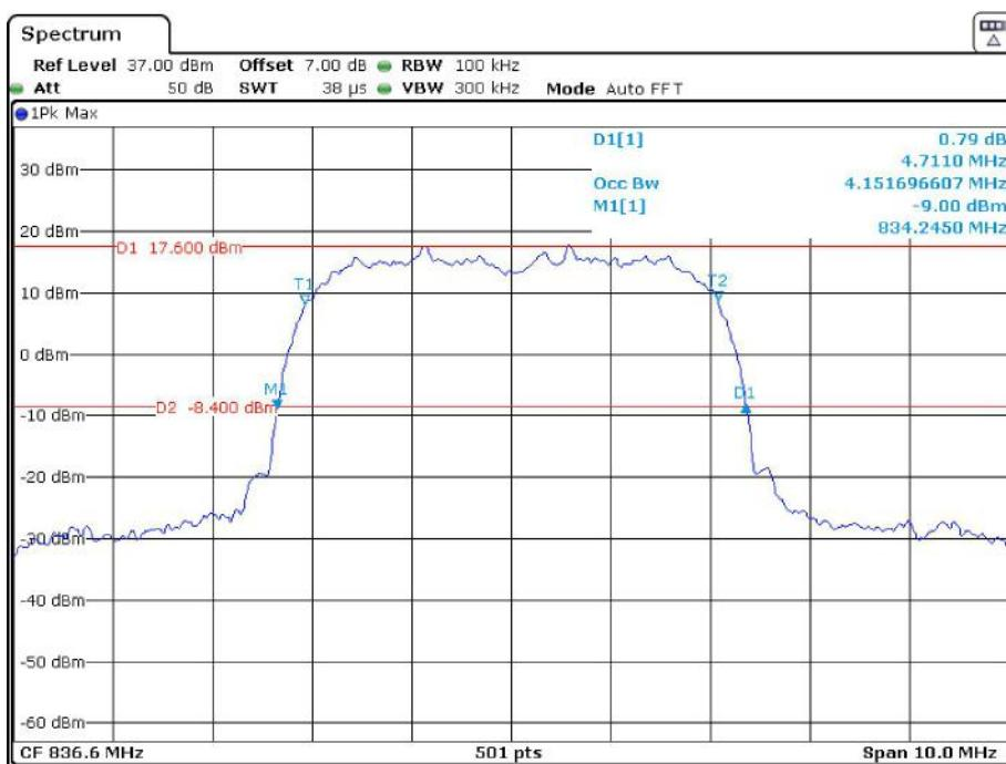
**26 dB Emissions &99% Occupied Bandwidth for HSDPA (16QAM) Mode, High channel**
