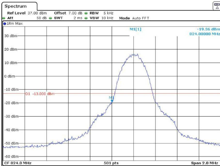
**Cellular Band, Right Band Edge for GSM (8PSK) Mode**
