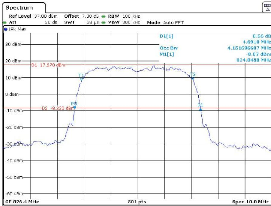
**26 dB Emissions &99% Occupied Bandwidth for HSDPA (16QAM) Mode, Middle channel**
