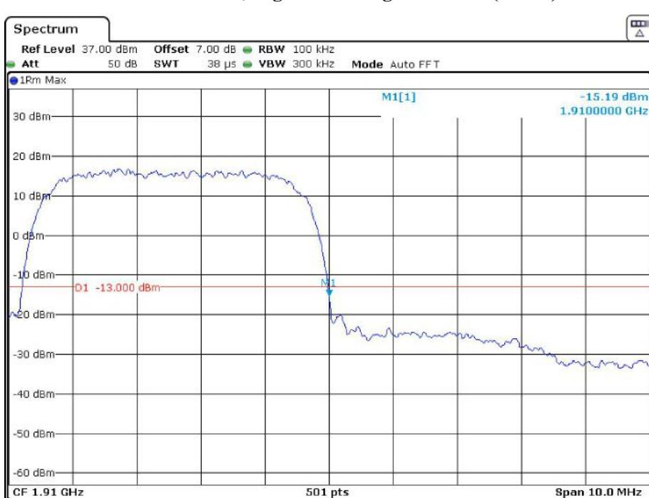
**PCS Band, Left Band Edge for HSDPA(16QAM) Mode**
