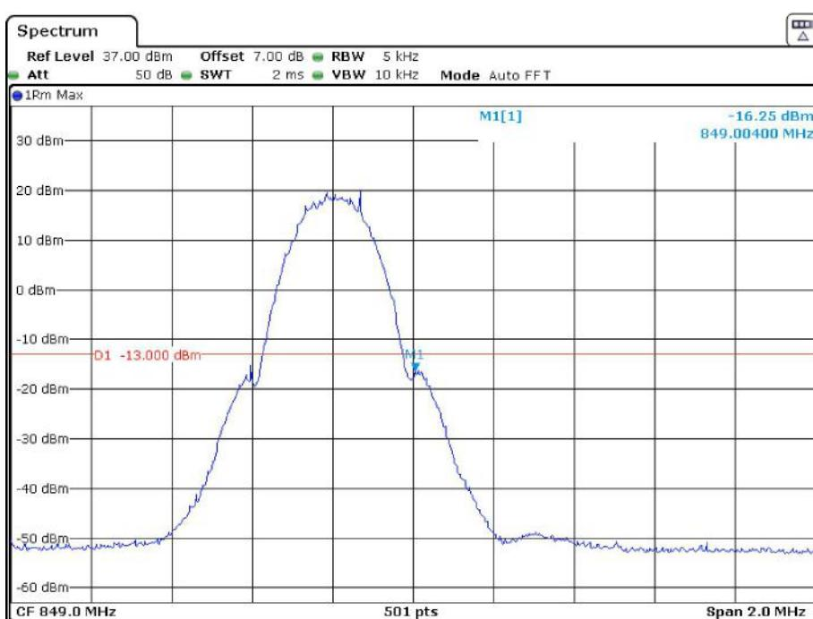
**Cellular Band, Left Band Edge for GSM (8PSK) Mode**
