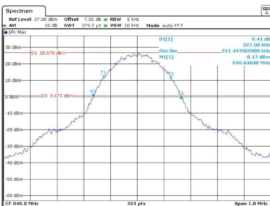
**26 dB Emissions &99% Occupied Bandwidth for RMC (BPSK) Mode, Low channel**
