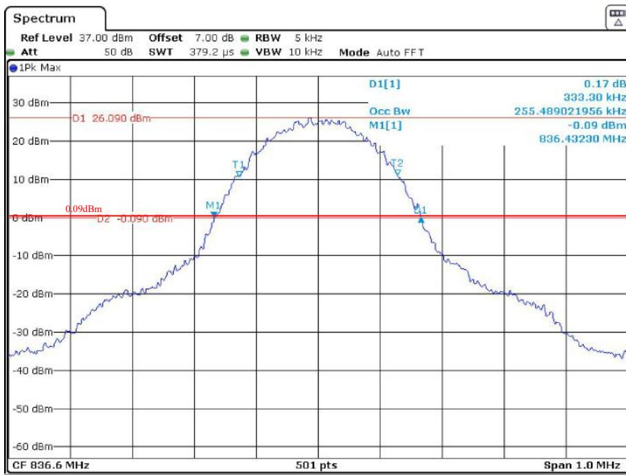
**26 dB Emissions & 99% Occupied Bandwidth for GSM(8PSK) Mode, High channel**
