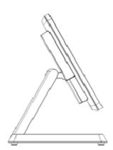
Single-screen 15 inch Device, W x D x H: 349 x 252 x 331, Main Display flip angle: 5-180°
