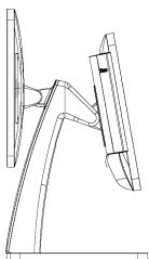
15.6-inch main screen + 15.6-inch secondary screen, length  $\times$  width  $\times$  height: 380mm\*205mm\*362mm; main screen flip angle 0-45°, secondary screen flip angle 0-30°
